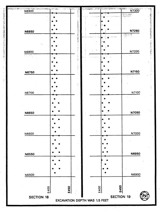
FIGURE 72 POST-REMEDIAL ACTION SAMPLING LOCATIONS ON THE CENTRAL DRAINAGE DITCH - SECTIONS 18 AND 19
