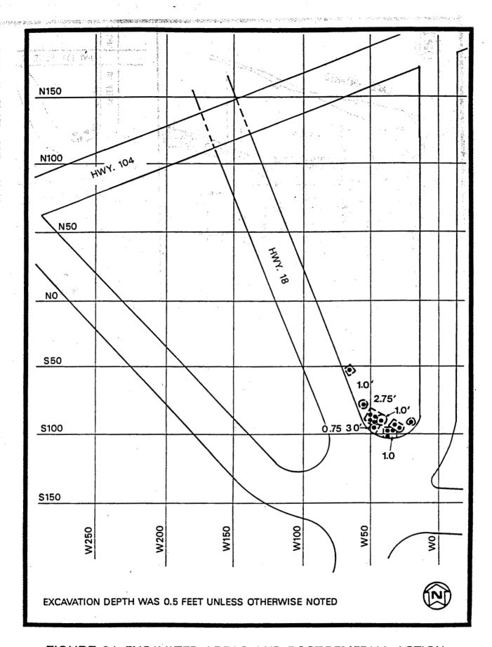
FIGURE 84 EXCAVATED AREAS AND POST-REMEDIAL ACTION SAMPLING LOCATIONS FOR ANOMALY AA
