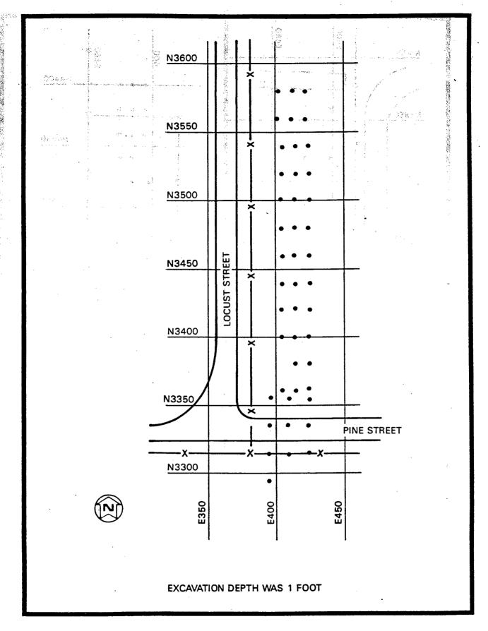
FIGURE 67 POST-REMEDIAL ACTION SAMPLING LOCATIONS ON THE CENTRAL DRAINAGE DITCH - SECTION 9
