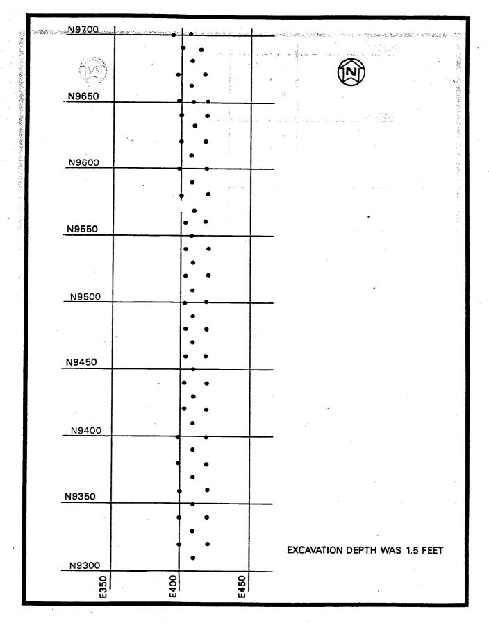
FIGURE 76 POST-REMEDIAL ACTION SAMPLING LOCATIONS ON THE CENTRAL DRAINAGE DITCH - SECTION 25
