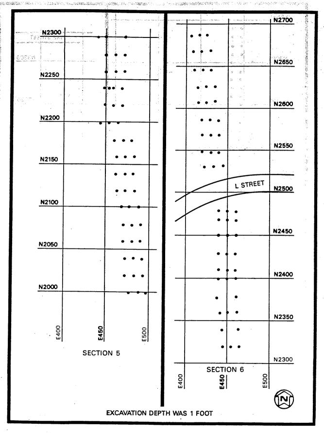
FIGURE 65 POST-REMEDIAL ACTION SAMPLING LOCATIONS ON THE CENTRAL DRAINAGE DITCH - SECTIONS 5 AND 6
