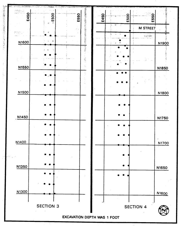
FIGURE 64 POST-REMEDIAL ACTION SAMPLING LOCATIONS ON THE CENTRAL DRAINAGE DITCH - SECTIONS 3 AND 4
