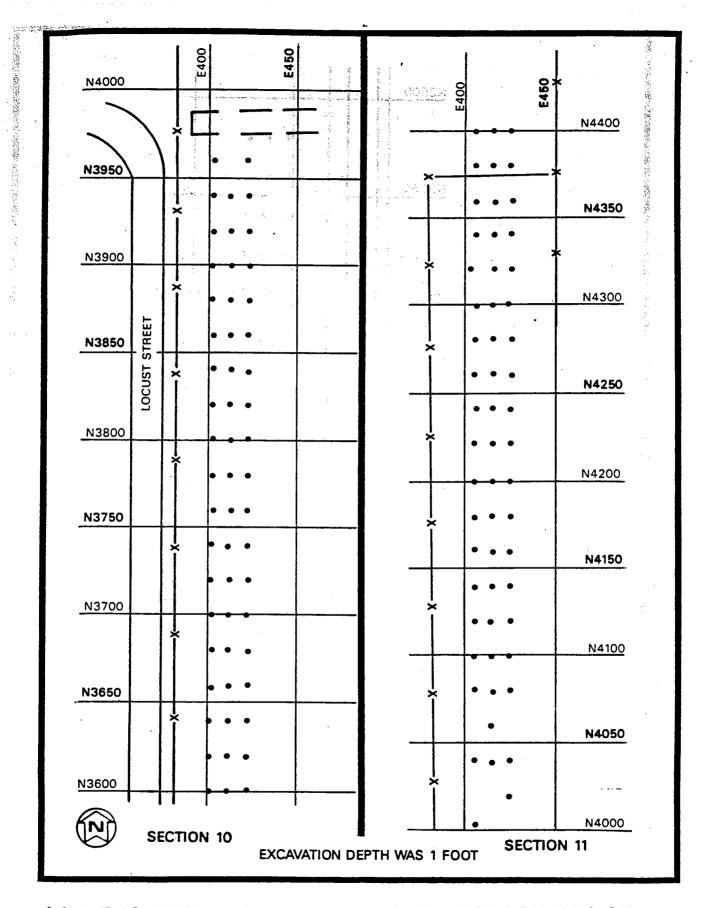
FIGURE 68 POST-REMEDIAL ACTION SAMPLING LOCATIONS ON THE CENTRAL DRAINAGE DITCH - SECTIONS 10 AND 11
