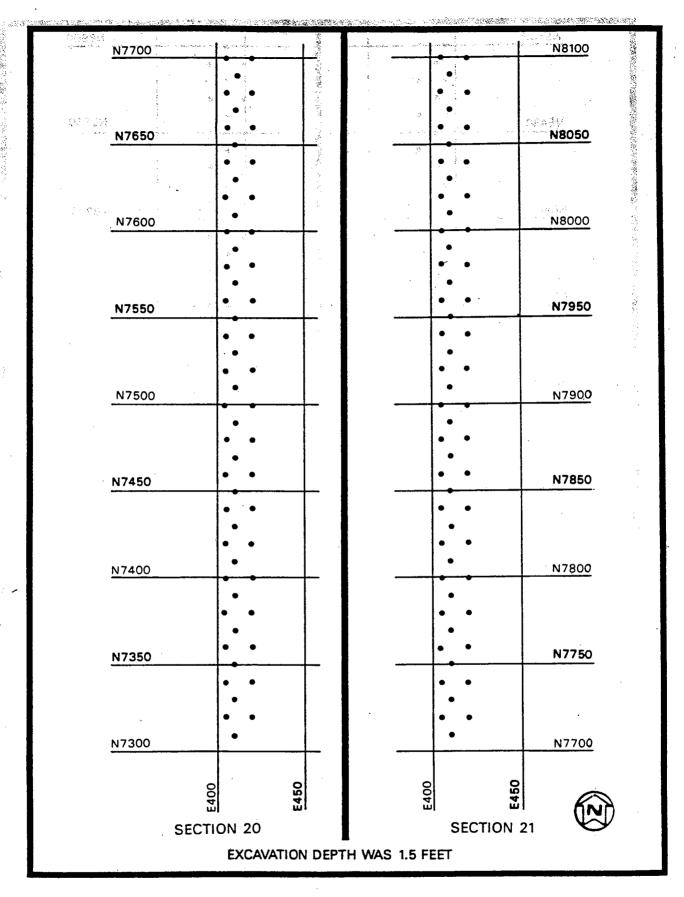
FIGURE 73 POST-REMEDIAL ACTION SAMPLING LOCATIONS ON THE CENTRAL DRAINAGE DITCH - SECTIONS 20 AND 21
